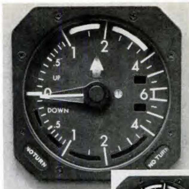
MODIFIED vertical speed indicator, CAS cockpit display by McDonnell Douglas, orders one plane (above) to climb; other, to dive. Each pilot limits the rate of climb or descent so that the pointer does not reach lighted area
